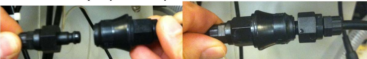
6. Connect the water supply line (the line going to the instrument is the male connector, the line to the furnace is the female connector with the sliding part). The connectors just push straight together
