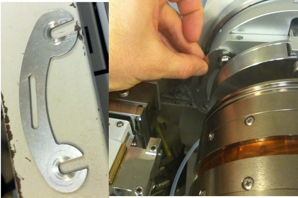
5. Connect the water return line (the line going to the instrument is the female connector with the sliding part, the line to the furnace is the male connector). The connectors just push straight together. You will have to use some force to get the connectors to click together. Make the connection quickly or water may leak out.
