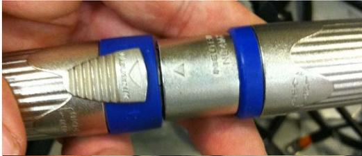
Connect the cables with these two triangles line up when connecting the power supply cable or disconnecting it. Gently twist the connectors, as shown, to lock the power supply cables together.
