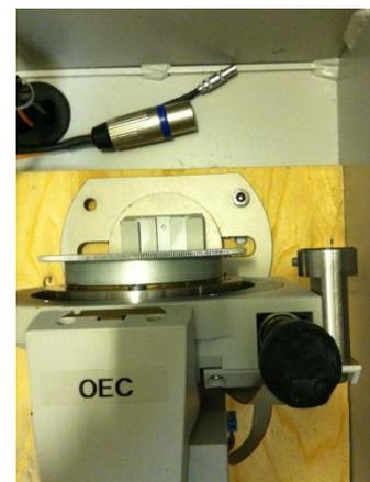
2. Put in the four hex screws that will hold the furnace in place (they go in the places where the black thumbscrews were that were holding on the OEC or sample spinner, circled in red in picture below). Tighten them until they are about  $\frac{1}{4}$  of the way into the hole. The screws are stored in the blue box on the left side inside the instrument hutch.
