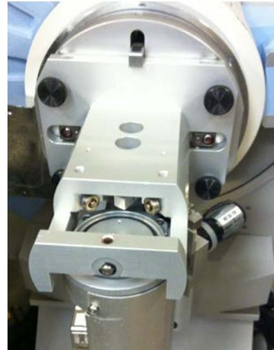
5. Use the four thumbscrews to tighten the stage into place
